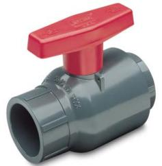
This industrial grade, quarter turn shutoff valve is popular where maintenance-free installations are desired for a variety of chemical processing, industrial and OEM applications. IPS Sizes 1/2" - 4" available with socket, threaded or flanged end connectors, 6" size available with socket or flanged end connectors. 6" valve uses high-efficiency lever style handle for easier operation
